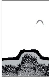
Structure is soft— probably a mud pile
